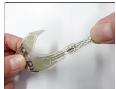
Stretchable FPC with Hydrogel
