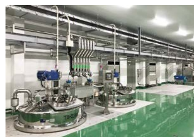
Yamasa Shiga Ryuo factory Production tanks and automatic raw material feeding equipment
